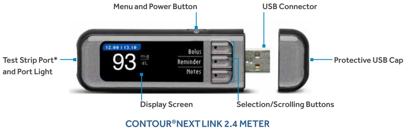
Your meter has a permanent rechargeable battery. **It is important that the meter be charged prior to your in-person training.** To charge your meter:
