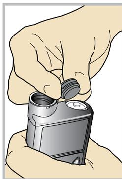
**STEP 2.** Place the battery cap onto the pump. Use the edge of the pump clip to turn the cap to the right (clockwise) and tighten until the slot is horizontal to the pump. See image below.
