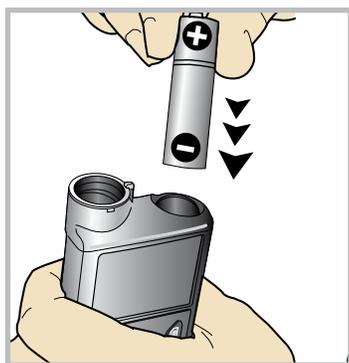
**STEP 1.** Place the battery into the battery compartment with the negative (flat) end going in first.
